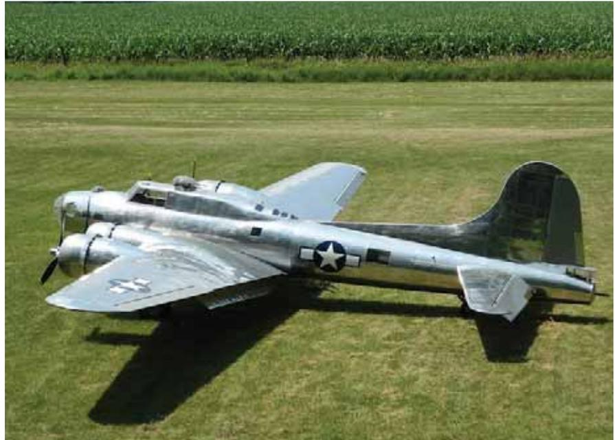
*Jack Bally's totally unique 1/3 scale B-17G is 25 feet long with a wingspan of 43 feet 7 inches and features retractable gear and working flaps. The fuel tanks hold 42 gallons and the estimated cruise speed is 110 knots.*
